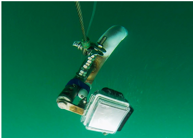
Figure 7. Version KLS 4.2. Photograph from tow cable mounted camera showing offset tow point and longline passing through setter.
