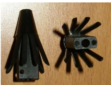
Figure 1: MiniPAT tag used for spinetail devilrays. Top: Tag showing the tag body (left) and tether (right). The main “umbrella” anchor with white dacron sleeves on some barbs is at the right hand end of the tether, and the secondary “tie-down” anchor is at the bottom of the yellow tubing. Bottom: Enlargement of two umbrella anchors showing eight nylon barbs (minus the Dacron sleeves).
