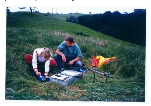
Plate 2 Taking readings with the LAI-2000 canopy analyser at stream level (B). A small plastic bottle was taped on the sensor 'wand' to avoid submersion.
