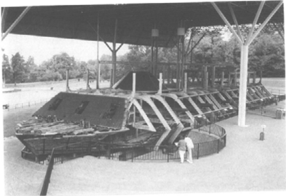
Figure 28 U.S.S. Cairo, a Union iron-clad river gunboat, sunk in the Yazoo River, Mississippi, in 1862. The boat was taken from the river in the early 1960s, and neglected for many years. It is now housed by the Vicksburg National Military Park under a roof, with destroyed parts of the structure "ghosted" with laminated wooden beams. The boat continues to have several conservation problems, partly because of its exposure to climatic fluctuations. Although periodically reimpregnated with sprayed polyethylene glycol (a water-soluble waxy alcohol which is designed to maintain the cell-structure of the original wood), its conservation status is not good.
