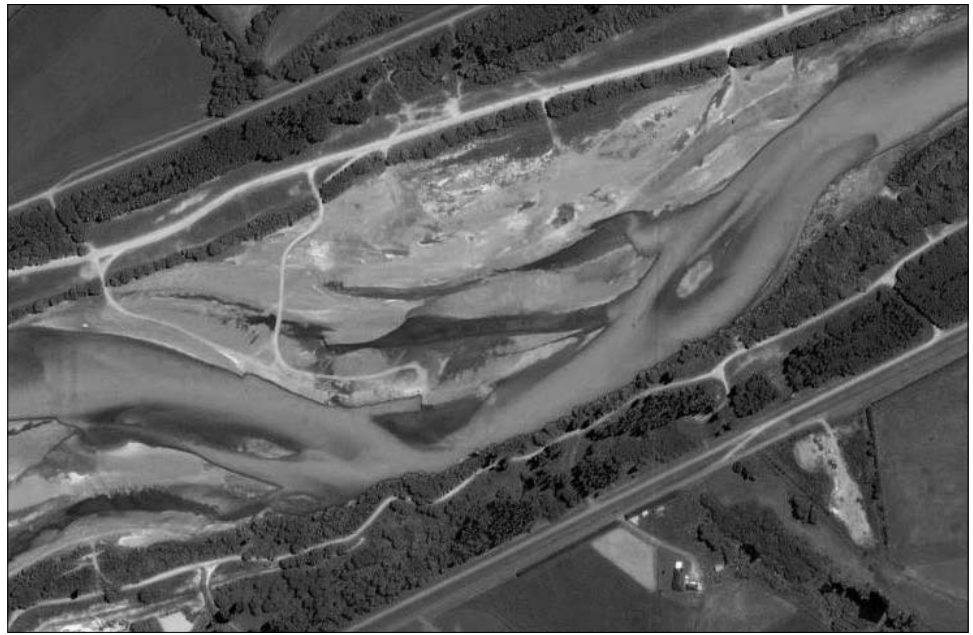
Figure A1.5. An impacted reach. The lower Waimakariri River, north of Christchurch, channelised by stopbanks.
