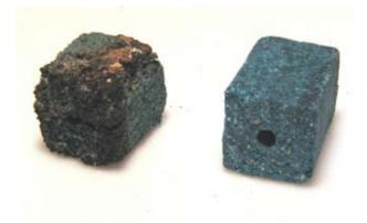
Figure A2.4B. Pestoff® bait weathered for 8 months (on left). Half the bait's surface was covered with brown and white mould. Some baits were slightly fragmented. Unweathered block on right for comparison.
