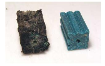
Figure A2.5A. Contrac® weathered for 12 months (on left). Most of the bait's outer surface was covered with brown mould, wispy white and powdery greed mould. Unweathered block on right for comparison.
