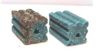
Figure A2.2A. Contrac® weathered for 3.5 months (on left). Approximately 50% of the bait's surface was covered with brown mould. Unweathered block on right for comparison.
