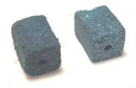
Figure A2.3B. Pestoff® bait weathered for 5 months (on left). The appearance of the bait was similar to bait weathered for 2 and 3.5 months. Unweathered block on right for comparison.
