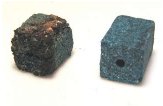
Figure A2.4B. Pestoff® bait weathered for 8 months (on left). Half the bait's surface was covered with brown and white mould. Some baits were slightly fragmented. Unweathered block on right for comparison.
