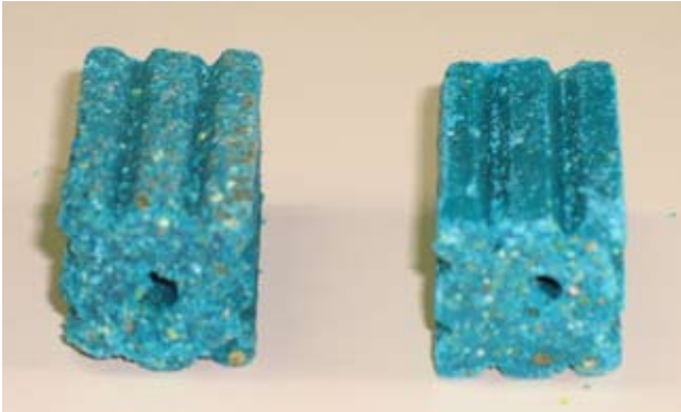
Figure A2.1A. Contrac® weathered for 2 months (on left). A small amount of brown mould was visible on the upper surface. Unweathered block on right for comparison.
