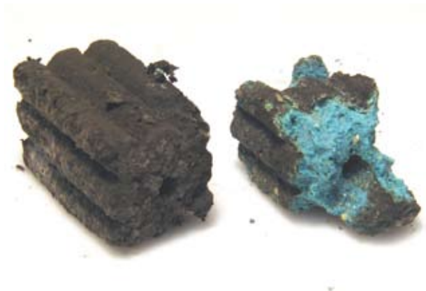
Figure A3.1A. Contrac® bait weathered for 12 months (on left) and after one night presented to a ship rat (on right). This photo demonstrates that the bait was only weathered on the surface and appeared similar in colour and density to fresh bait once the weathered surface was removed.
