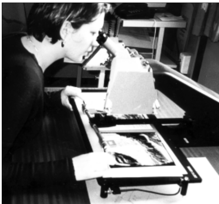
Figure 3. An illustration of the use of mirror stereoscope. Model: Wild Heerbrugg Type 369275 Switzerland.
