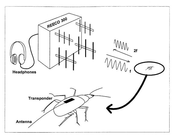
FIGURE 6. REECOTM MODEL 300 HAND-HELD TRANSCEIVER UNIT WITH HEADPHONES AND EXAMPLE OF A SMALL TRANSPONDER (HP2835 DIODE AND 3 cm ANTENNA) GLUED TO THE BACK A CARABID BEETLE.
