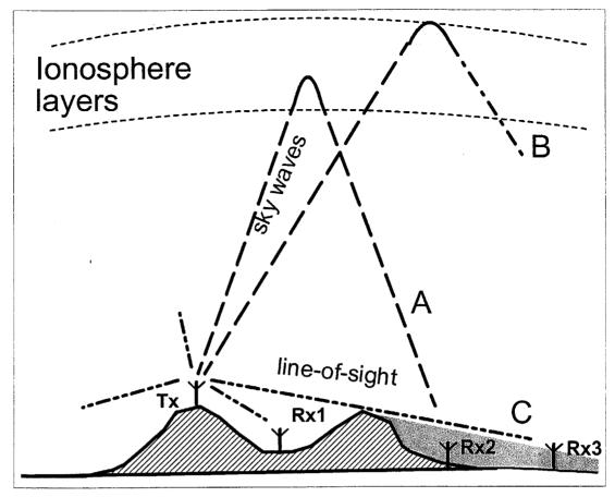
FIGURE 2. RADIO SIGNAL PROPAGATION: EXAMPLE OF HF SKY WAVE PROPAGATION (A & B) FROM Tx TO Rx1-3 AND VHF LINE-OF-SIGHT PROPAGATION (C) FROM Tx TO Rx1 AND Rx3. Rx2 REMAINS IN TOPOGRAPHIC SHADOW TO VHF SIGNALS.
