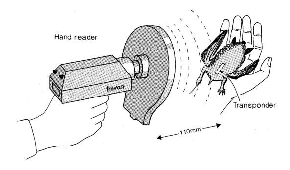
FIGURE 5. TROVAN HAND READER AND SHORT-TAILED BAT, SHOWING TRANSPONDER IMPLANT SITE.
