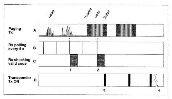
FIGURE 3. TRANSPONDER ACTIVATION TIMING. TRANSPONDER'S RECEIVER (Rx) POLLING EVERY 5 s (B) RESPONSE TO NOISE (C, 1) AND VALID PAGING TRANSMITTER (Tx) CODED SIGNAL (C, 2). TRANSPONDER'S TRANSMITTER ACTIVATED (D, 3) AND PULSES UNTIL TURNS OFF (D, 4) AFTER A SET DELAY.
