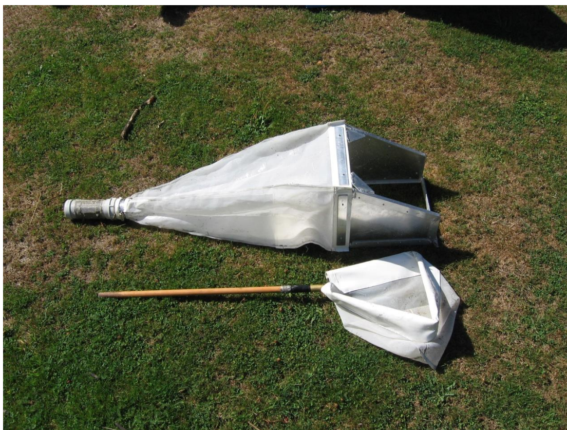
Figure 1. A Surber sampler (top) and kick-net. Note framing around the base of the Surber sampler to isolate a known area of stream bed, side walls to direct current, and receptacle to concentrate sample. Photo: Tanya Blakely.
