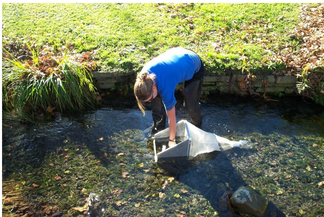
Figure 2. Collecting the Surber sample. Note the operative stands adjacent to or downstream of the sampler. Photo: Duncan Gray.
