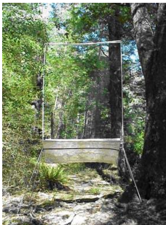
Figure 2. A harp trap—designed specifically for trapping bats.
