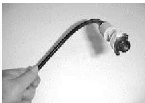
Figure 6. Small video camera and infrared light source used for inspecting bat roosts. Reproduced from Reardon (2001).
