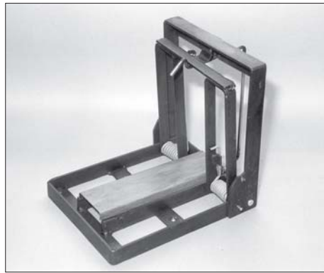
Figure 1. Waddington backcracker trap showing: set position with bars upright (left); and triggered position with bars down (right).
