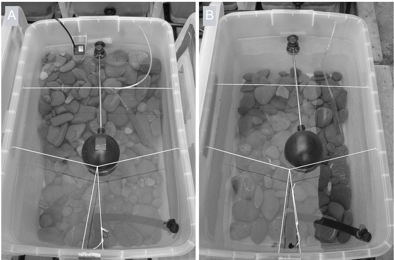
Figure 7. Examples of treatments in the holding conditions: A. an angled substratum, water current treatment tank, showing extra substratum; and B. a flat substratum, no water current treatment tank. Submersible pump, air diffuser, ball cock, stand pipe and tensioning cords common to both.
