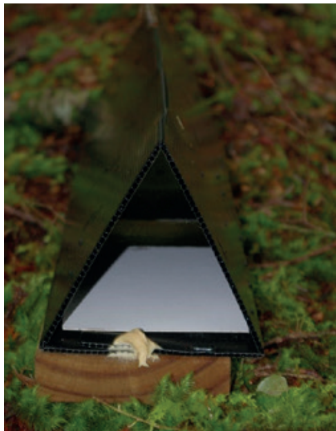
Figure 4. Tracking tunnel containing a pre-inked card.
