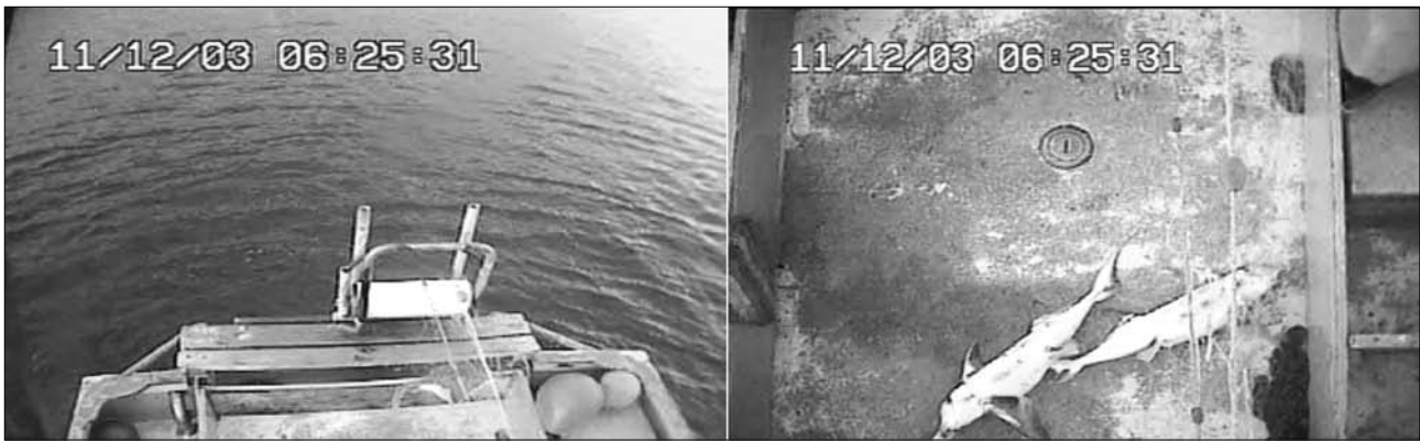
Figure 2. An example view from the twin camera system mounted on a set net vessel. The photo on the left is through a wide-angle lens (3.6 mm) and that on the right is through a low-magnification telephoto lens (6 mm). Note that while these images are reproduced in black and white, the real images are in colour.
