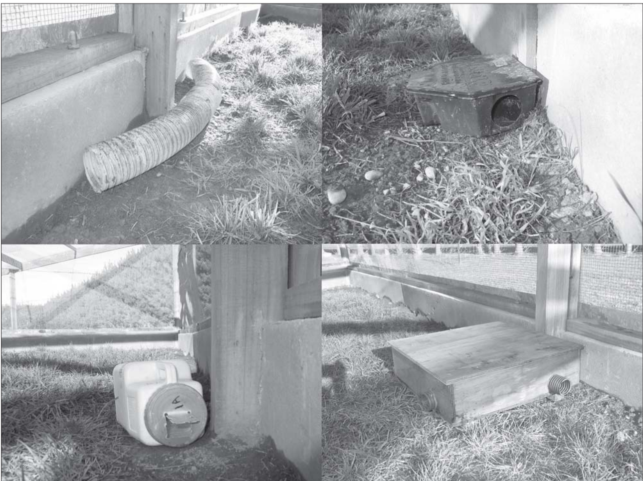
Figure 1. Bait station types as set up for testing Norway rat preference (left to right, top then bottom): yellow plastic pipe, black plastic box, white plastic bottle, and wooden motel.
