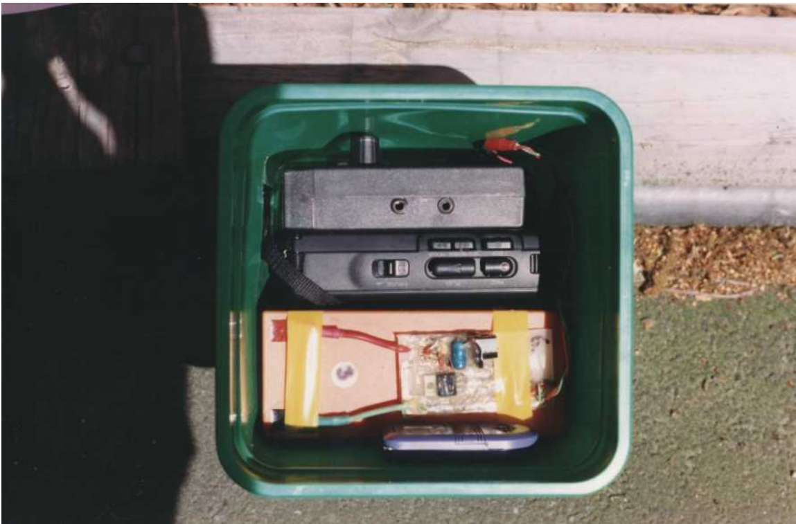
Figure 1. (A). Components of the bat detector system: 1, bat detector; 2, gel battery with voltage reduction circuit; 3, voice activated tape recorder; 4, talking clock. (B). Components fit into a four litre plastic container.
