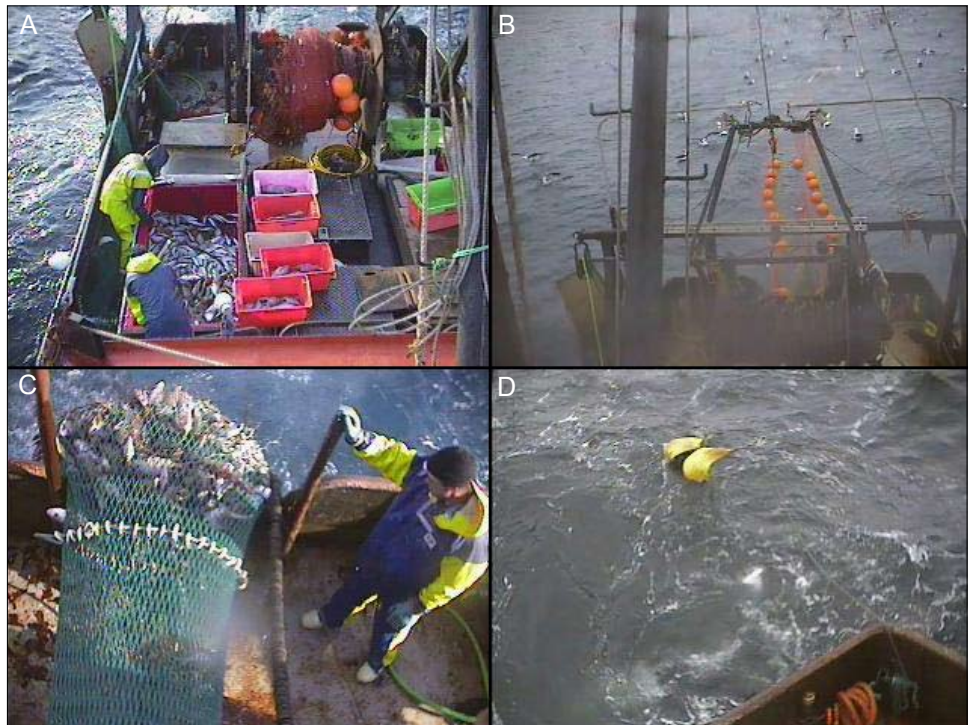
Figure 4. Sample images from V2. A. View used for analysis of offal discharge, discarded bycatch and protected species bycatch. B. View used for assessing seabird abundance and mitigation device deployment. C. View used to detect protected species bycatch when the codend was hauled over the stern. D. View initially set up to detect warp strikes. This view was eventually used to detect deployment of the warp scarer that was clipped to the main warp.
