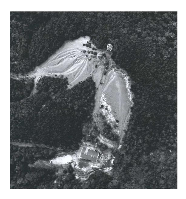
Frontispiece. Near vertical aerial view of the poppet head, mullock heap, reconstructed engine shed and the head of the aerial cableway. Note the drain around the flat and the pattern of erosion on the mullock heap.
