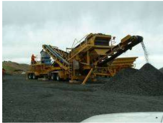
Figure 1; Example of mobile aggregate screening and crushing plant (photo supplied by MDL)
