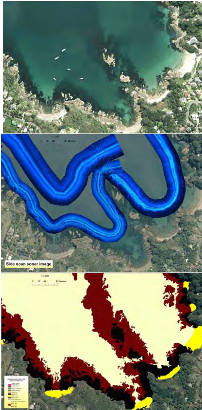
Figure 4. Aerial photograph (Auckland Council, top), side scan swath (centre) and GIS habitat map for Hekerua Bay.
