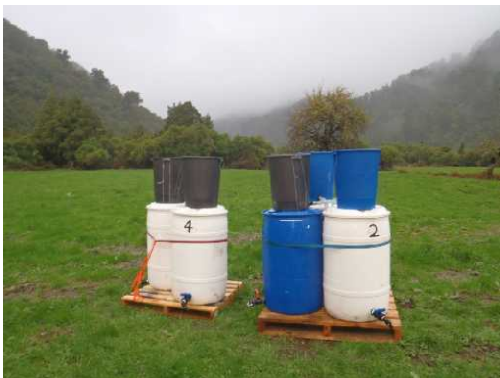
Figure 10: Field leach columns for Te Kuha rocks
