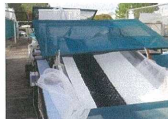
NIWA's experimental ramps to test fish swimming abilities (source NIWA)
