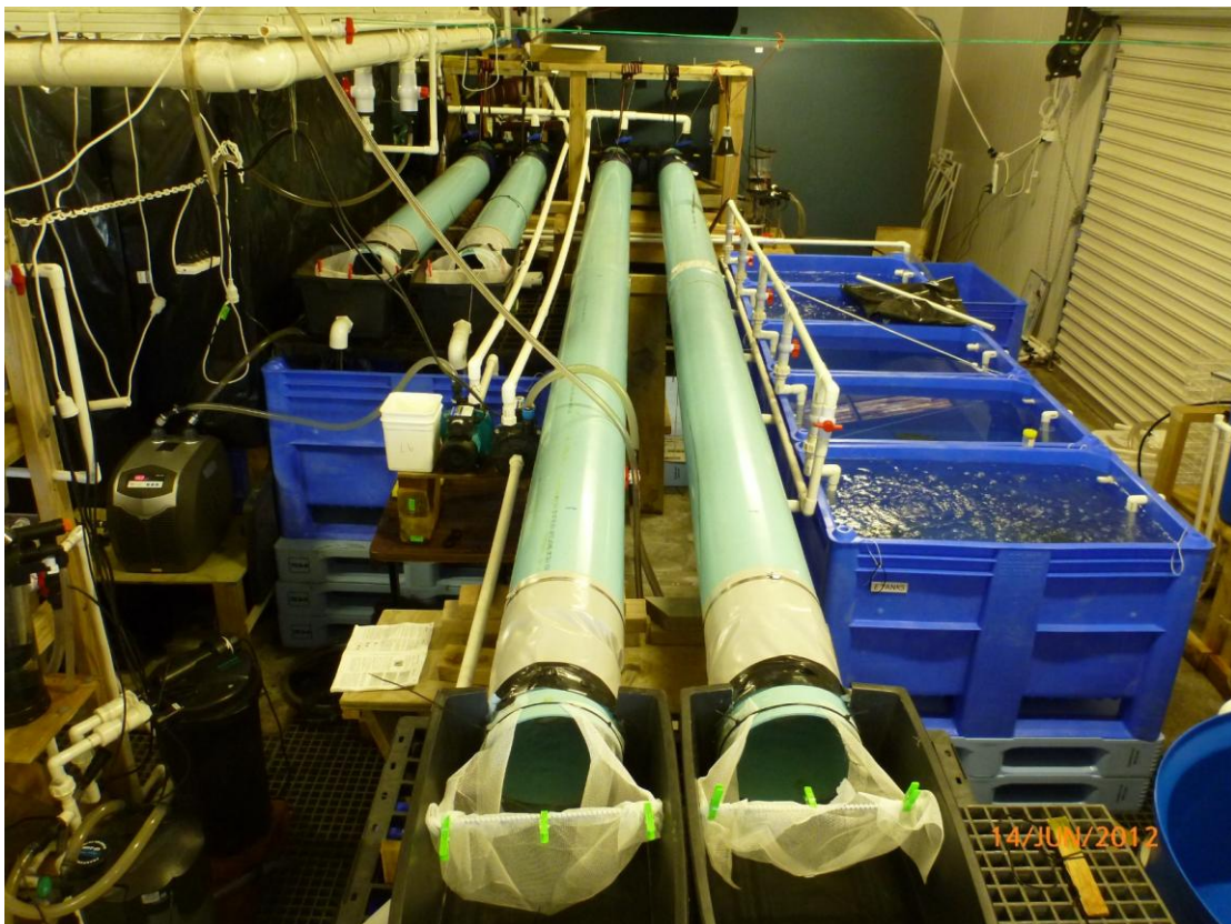
Figure 4: Paired experimental set-up for testing passage success of fish and shrimp through 3m and 6m culvert pipes with and without ropes and at varying gradients and flows.
