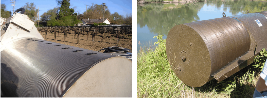
a. Internal brush projecting through the screen.
