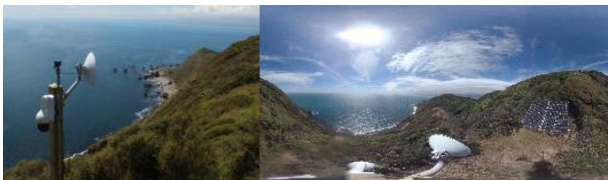
Figure 4-2: Kapiti Island fixed station telemetry site. A Garmin Virb 360° camera was integrated into the existing telemetry site at northern end of Kapiti Island overlooking the marine reserve (left) giving images (example right).
