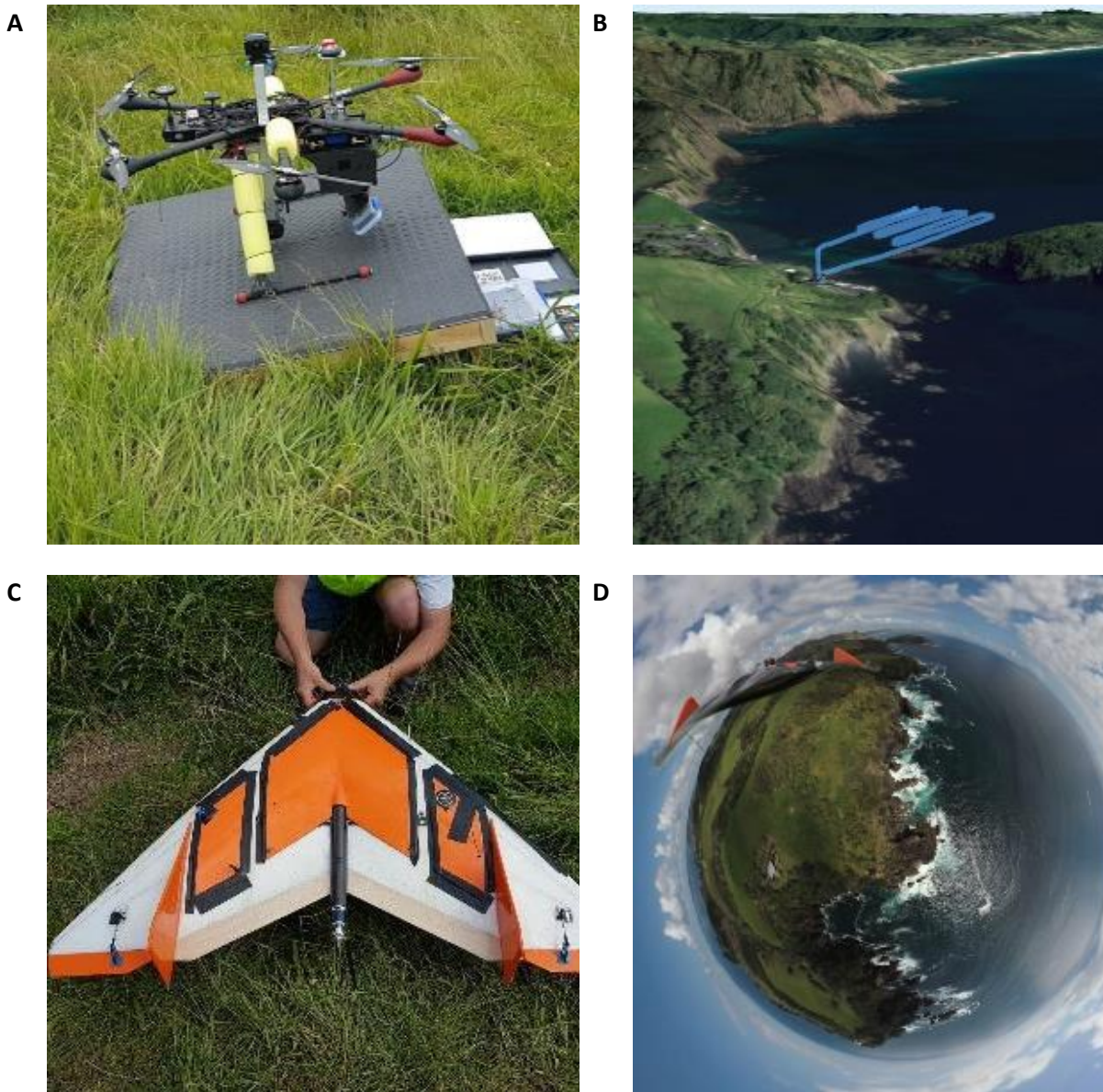
Figure 4-1: Testing radiometric measurements from drone at Leigh Marine Reserve, Cape Rodney. (A) Hexacopter drone (X-Craft) showing central top and bottom Garmin Virb 360 cameras and black active gimbal (with GoPro Hero 4, Micasense RedEdge, and Ocean Optics hyperspectral radiance sensors) pointing at 40 degrees from nadir. Calibration plates are in front of sensors to bracket pre-flight and post flight data. (B) One coastal habitat mapping survey track in Google Earth between Goat Island and Leigh Marine Reserve. (C) Valkyrie fixed wing drone (X-Craft) with Garmin Virb 360 inserted into nose. (D) One image example from Valkyrie drone video footage.
