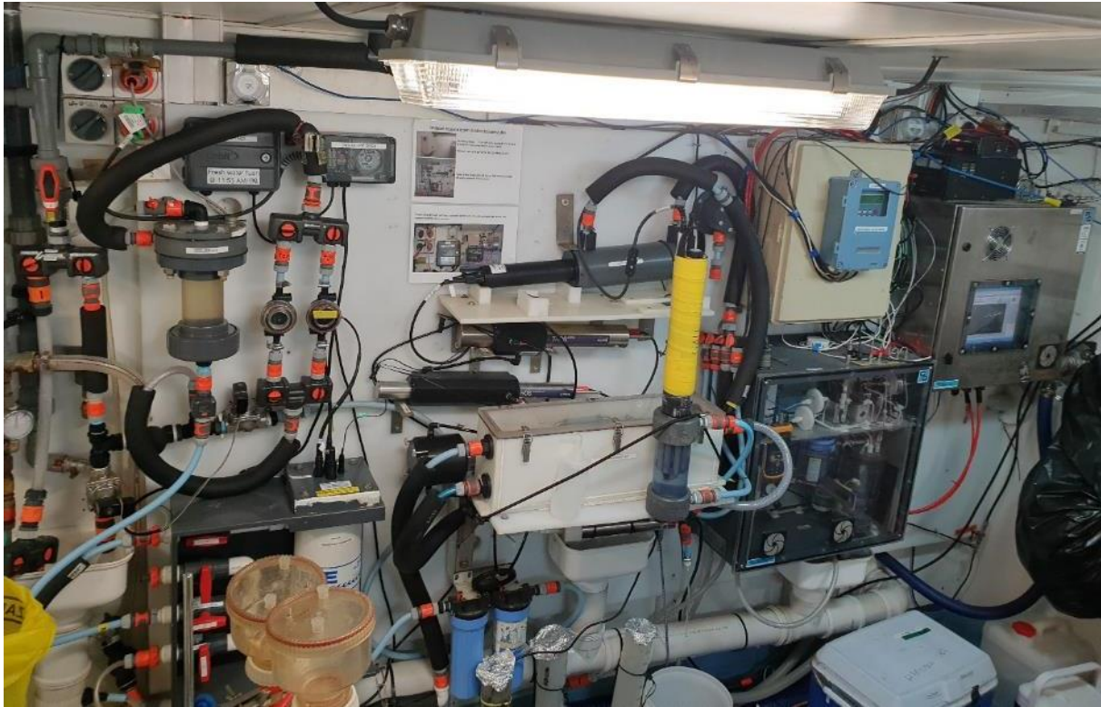
Figure 4-4: RV Tangaroa Underway Flow Through System (TUFTS) on voyage TAN2101. Image shows pre-screening sieves and vortex debubbler, prior to flowing through a series of in-line sensors including for attenuation and sediment backscatter. A simplified setup could be used on smaller research vessels and ships of opportunity like ferries and fishing boats. Source: O’Driscoll et al., (2021).
