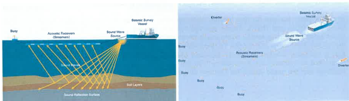
Figure 2: Schematic of 2D (left) and 3D (right) Marine Seismic Survey
