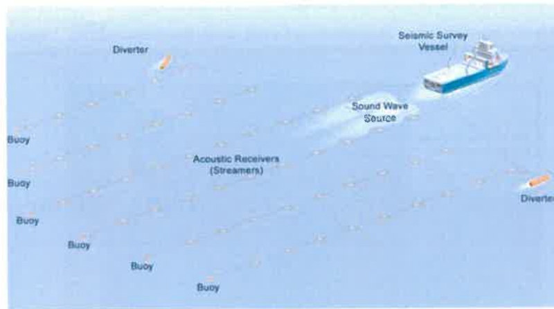
Figure 3: Schematic of acoustic sound waves being reflected from subsurface layers
