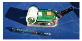
This GPS phone tag collects detailed location, temperature, dive and haulout data. A large battery (at left) enables the device to be used in the field for up to 6 months. This tag was made by the Sea Mammal Research Unit, University of St Andrew, Scotland.
