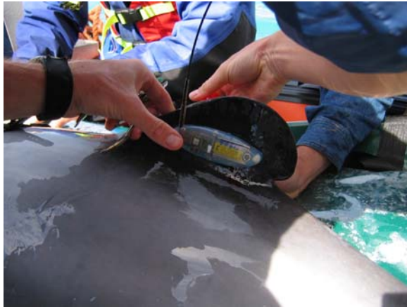
Figure 3. SPOT-3 tag on Hector's dolphin dorsal fin using two-pin attachment.
