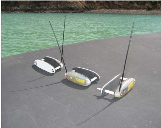
Figure 1. SPOT-3 tags with attachment pins and backplates.
