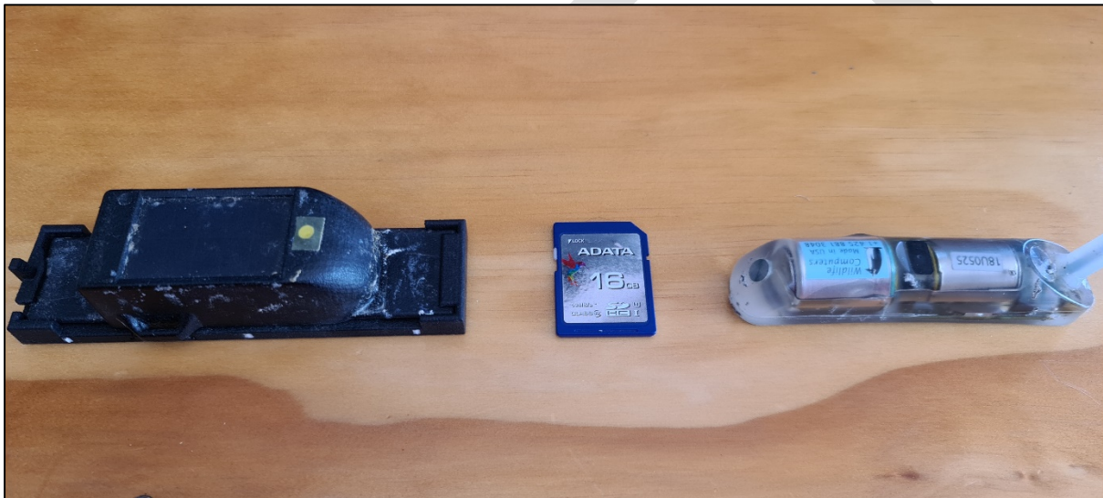
Figure 2. Transmitting devices used during four deployments in this study. Ornitrack-25, GPS-GSM dive transmitter (left) and Wildlife Computers SPOT-275 satellite transmitter (right); SD card shown for scale. Note that the Ornitrack-25 is sitting on a magnetized base plate that keeps the unit in sleep mode; the unit is deployed without this base.
