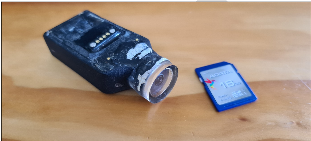
Figure 3. Animal-borne camera logger deployed on some hoiho during the course of this project. SD card shown for scale.
