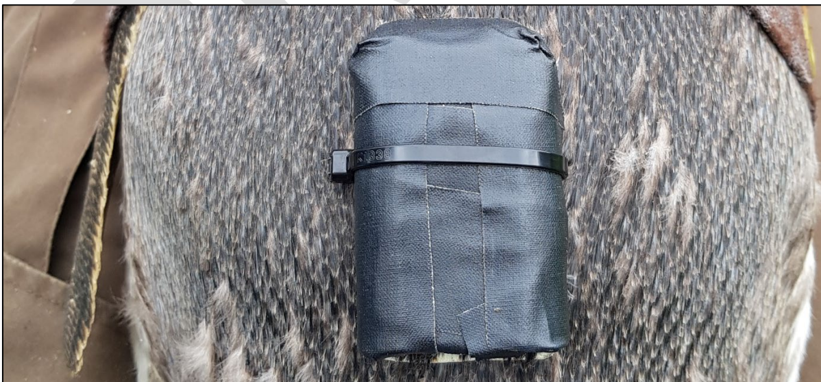
Figure 5. GPS dive loggers attached with tape and a cable tie to the lower back of a hoiho.
