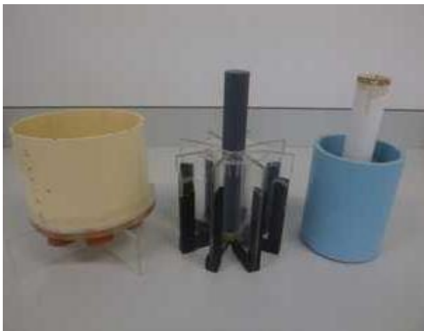
The 8-way sample splitter. L to R: bucket with eight bunged holes in the base, eight-vane plunger and weighted (5.6 kg) collar.
