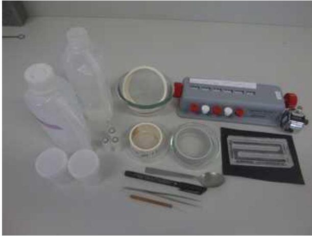
Equipment used included: squirt bottles of ethanol and water, small sieves, various containers, counters, Bogorov tray, forceps, petri dishes.
