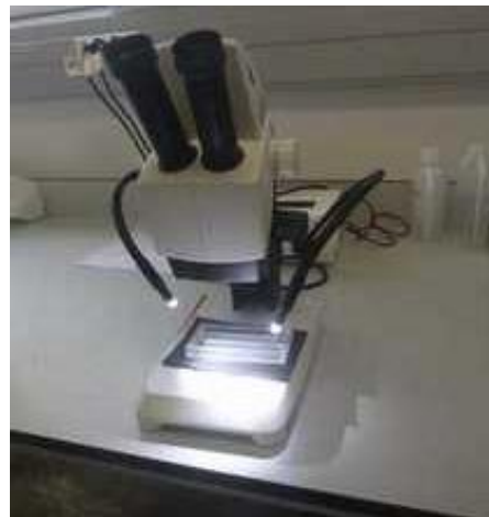
Leica EZ4W microscope with external lighting, Bogorov tray with black paper underneath.
