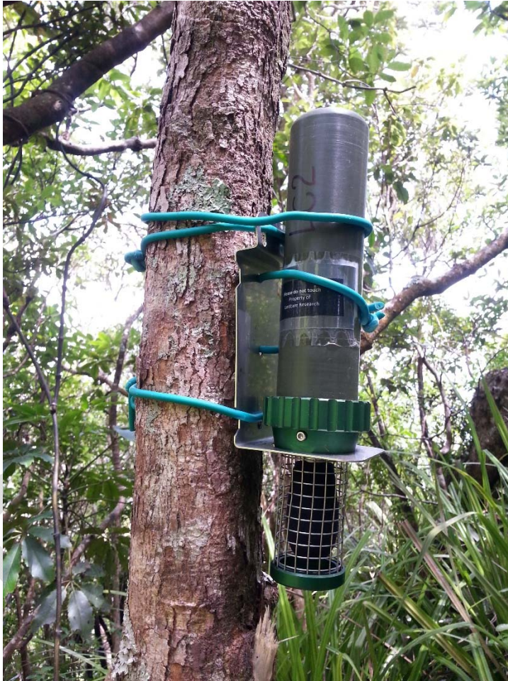
Figure 1 Example of the Department of Conservation automated acoustic recording unit deployed on the Moehau range, Coromandel, 2015/16.
