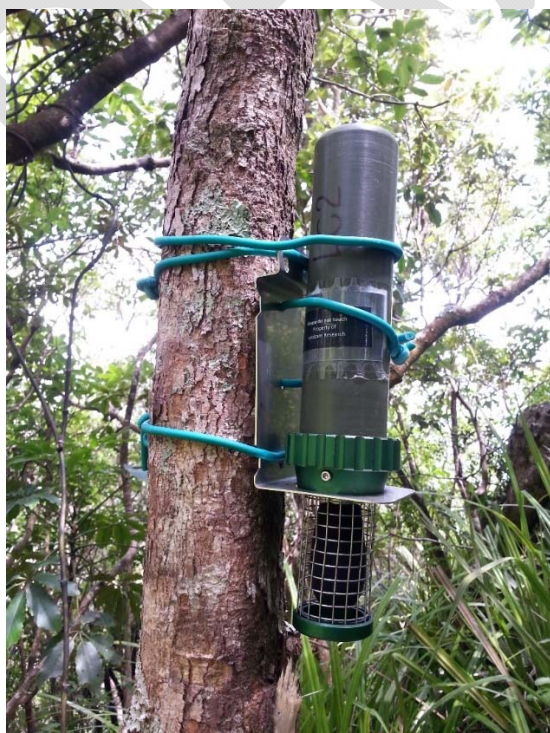
Figure 4 Example of the automated acoustic recording unit deployed on Hauturu-o-Toi/Little Barrier Island, 2015/16.
