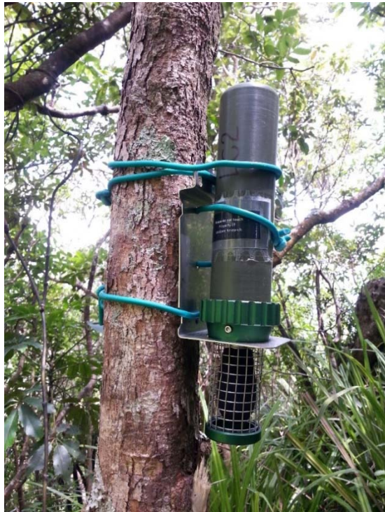
Figure 3 Example of the automated acoustic recording unit deployed on Great Barrier Island/Aotea, 2015/16.
