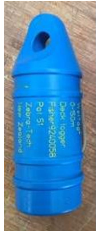
Figure 1: Current Zebra-tech Wet Tag design.
