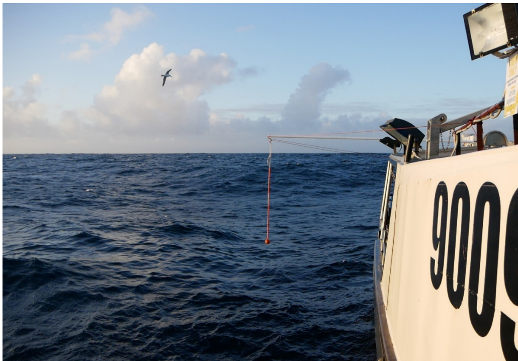
Figure 3. Photograph looking aft from in front of the hauling station on Vessel C, showing hauling mitigation device in place. Camera position was astern of the second light on the top of the shelter.
