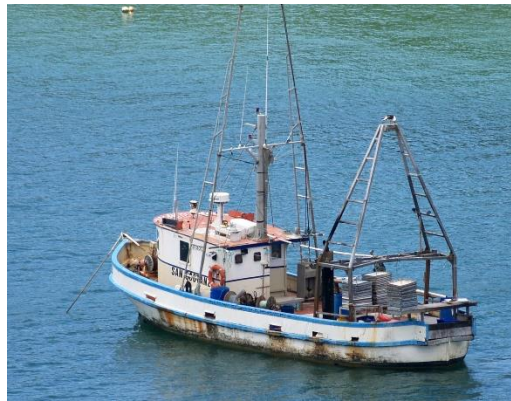
Figure 3. A former trawler that has been converted for inshore bottom longlining. The residual gantry metalwork in place provides many options for the attachment of tori lines. Photo: D. Goad.
