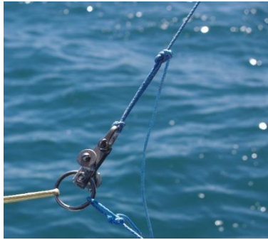
Figure 1. The variable tension link used during at-sea tori line trials.
