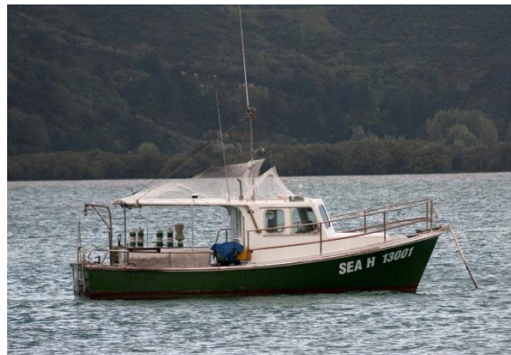
Figure 1. A small bottom longline vessel that is low to the water and has minimal deck structure at the stern for the robust attachment and effective elevation of a tori line. Photo: D. Goad.
