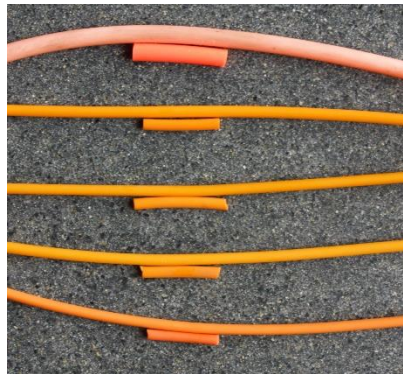
Figure 6. Five streamer materials after seven months exposure to ambient exterior conditions. The small segments are the same materials pre-exposure. The 9-mm diameter Kraton-like material is at the top, and T061 – T064 are in order from the second to top to the bottom of the figure.
