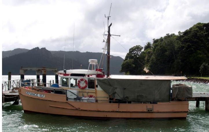
Figure 2. An example of a “typical” small bottom longline vessel, i.e., vessels 12-15 m in length with a shelter deck and some metalwork close to the stern. Photo: D. Goad.
