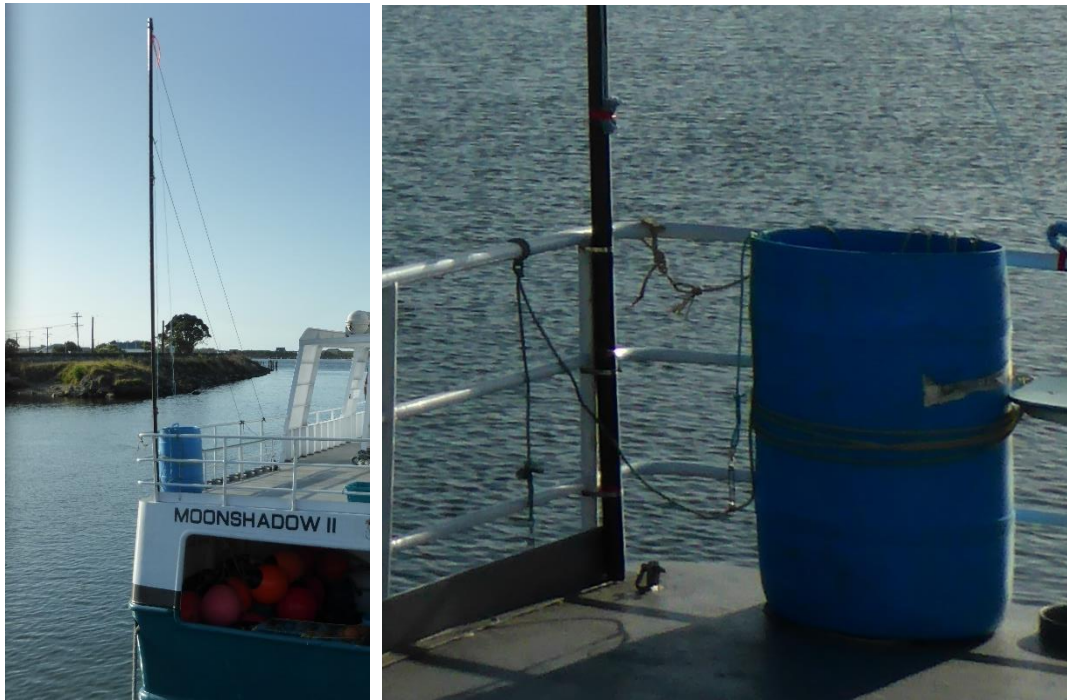
Figure 19. The tori pole attachment, and tori line storage drum, shown in context and close up on the FV Moonshadow.
