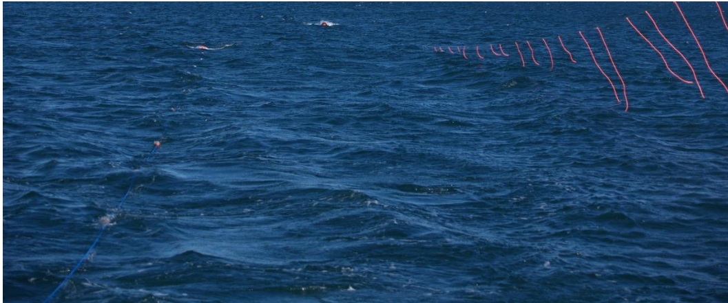
Figure 10. Tori line 8 showing the large road cone comprising the in-water section and the splash it created at 4 knots. The rope used to measure aerial extent (marked with floats at 5-m intervals) is visible on the left.
