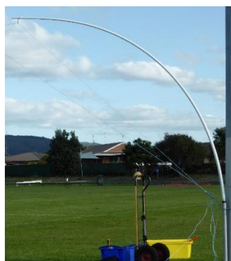
Figure 3. A tori pole under 20 kg of drag - more than was ever required to achieve an aerial extent of 80 m during the on-land trials.
