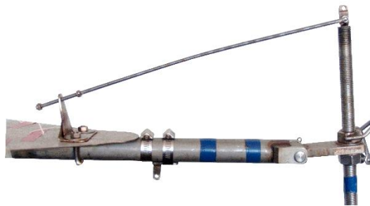
Figure 15: Photograph showing adjustable stop to control the amount of movement in the hinge at the forward end of the setter.
