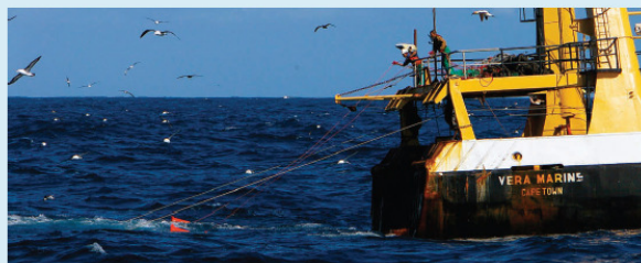
Crew deploy tori lines from a South African trawler. Tori lines have been developed by fishermen and scientists to reduce seabird deaths on trawl and longline gear. Photo: J. Pierre.
