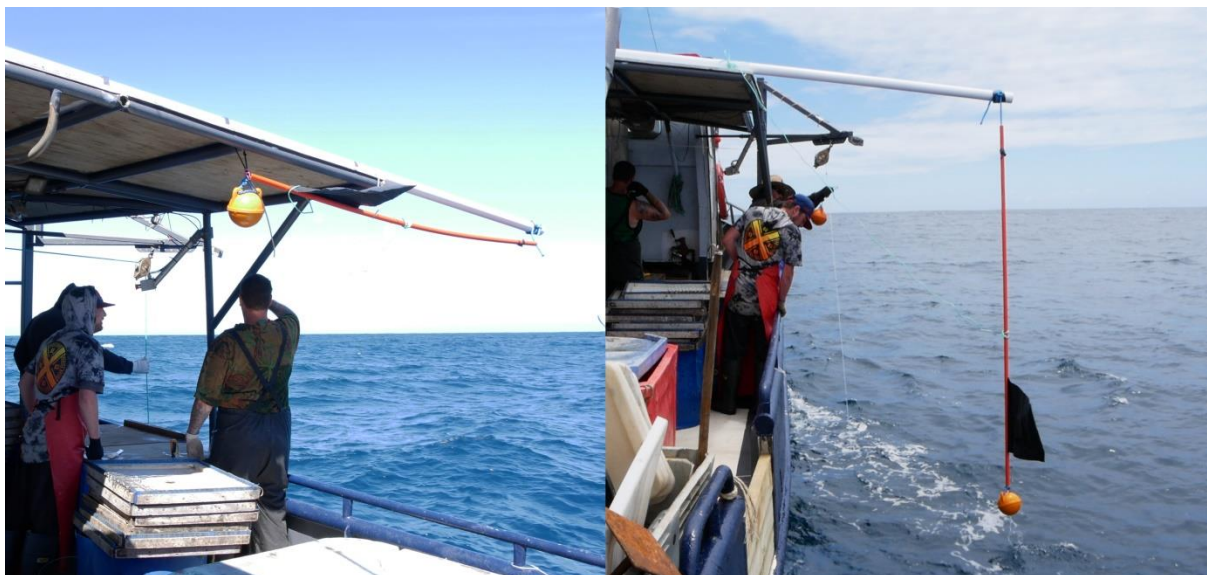
Figure 3: Photographs showing dangler stored on the underside of the shelter deck and deployed beside the vessel.
