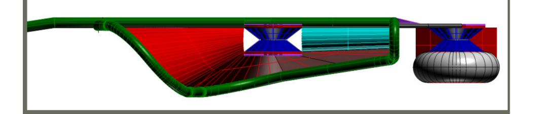
Rear roller is used to keep line in when weights go though the system, may require modifications to current weights, based on Dave Kellian's advice. Roller detail. Cheeks are made of plastic, with 4mm thick rubber centre disk to grip backbone.
