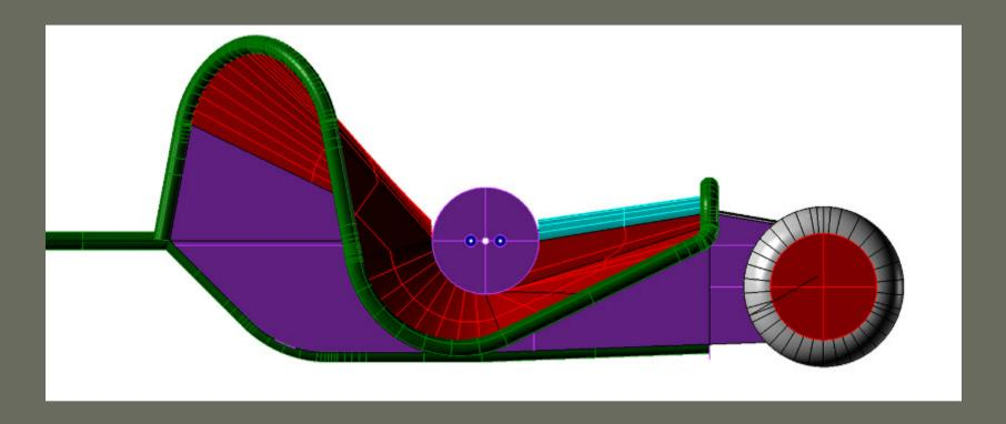
Rollers have teeth & rubber insert to improve traction on mainline. Also has ability to connect the rollers so that they are always driven
