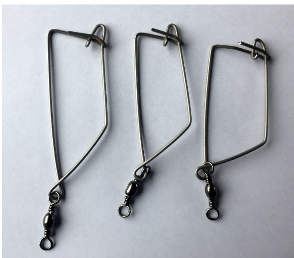
Figure 14. Photograph showing fourth clip design, note loop at top allowing it to spin freely on mainline
