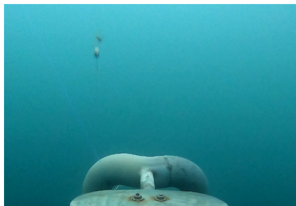
Figure 25. Pilchard bait damage as hook gets pulled forwards into setter – note bait still on the hook and a piece of loose guts above.
