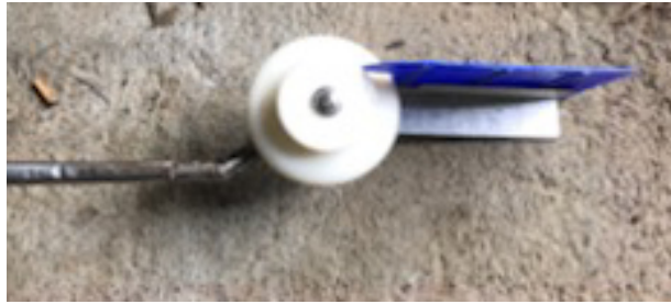
Figure 15. Photograph showing paravane added behind the wheel.
