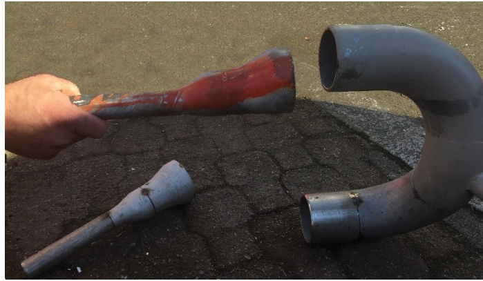
Figure 23. Photograph showing modifications made to the setter guide, with the shorter and larger diameter legs welded on, and the old legs removed.
