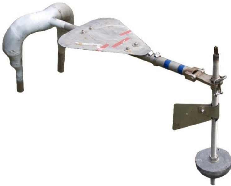
Figure 4. Schematic diagram and photograph of the underwater setter with a guide, at the start of the project.
