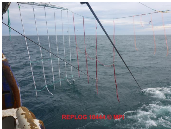
Figure 9. The Prototype III baffler viewed from the starboard stern quarter. The port warp has crossed the centre of the vessel and is protruding significantly from the protected area covered by the baffler's stern curtain.
