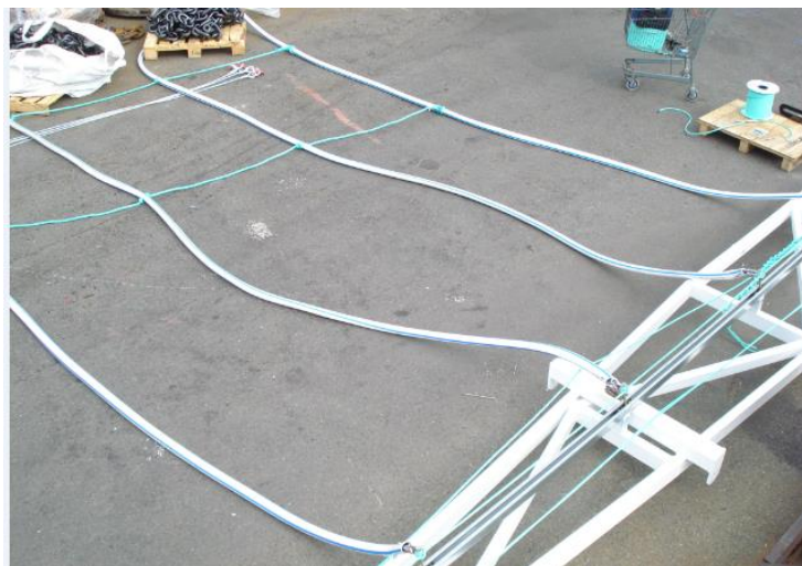
Figure 5. Assembly of the baffler dropper system using rope passed through plastic hose, to be deployed on the starboard side of the vessel.
