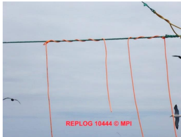
Figure 8. Kraton-like plastic noodle droppers from the stern curtain tangled around the curtain's top rope. (Note that following at-sea testing, these noodles were replaced by hose to prevent future tangling).
