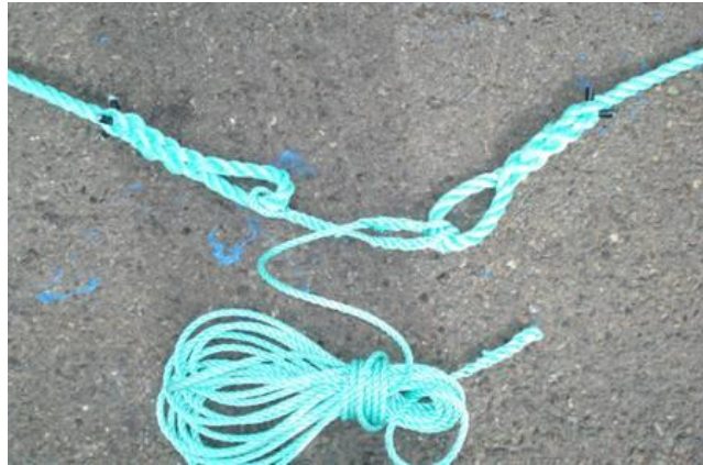
Figure 6. The weak link included in the stern curtain to allow the curtain to break into two parts should one of the booms be damaged or lost into the sea.
