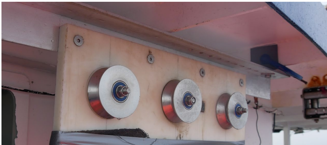
Figure 3. Photograph showing tension meter setup.
