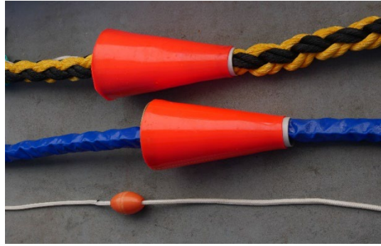
Figure 4. Photograph showing details of the tori line drag sections tested: 52 mm diameter 8 plait rope threaded through a 280 long 150 mm diameter cone (top), 32 mm rope covered in hose with the same cone (middle), and 9 mm trawl braid with a gillnet float (bottom).
