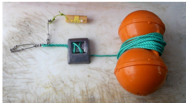
Figure 1. Modified 150 mm diameter floats with TDR housing attached, ready for deployment.
