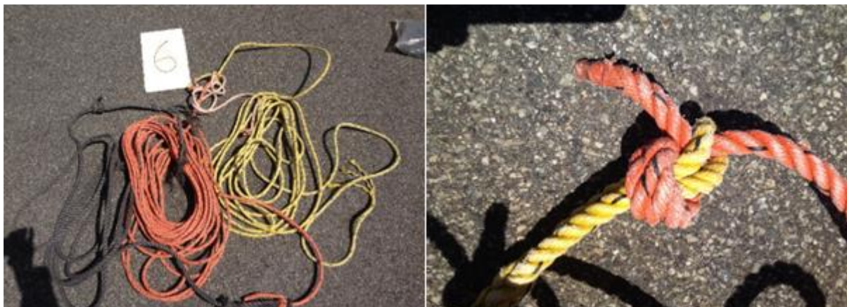
Figure 39. Recovered gear from a whale entanglement in Western Australia, illustrating (L) the three sectional ropes (black, orange and yellow) comprising the mainline, and (R) the join used to combine sectional ropes.
