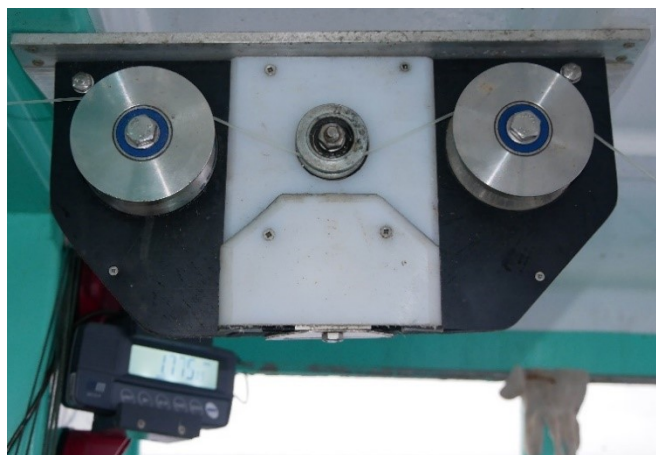
Figure 2. Photograph showing tension meter setup.
