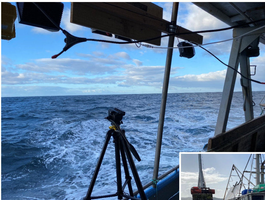
Figure 8. Light array on the starboard side of the Southern Cross used in May 2021. Tripod for thermal imaging scope cable-tied to the rail of the boat.
