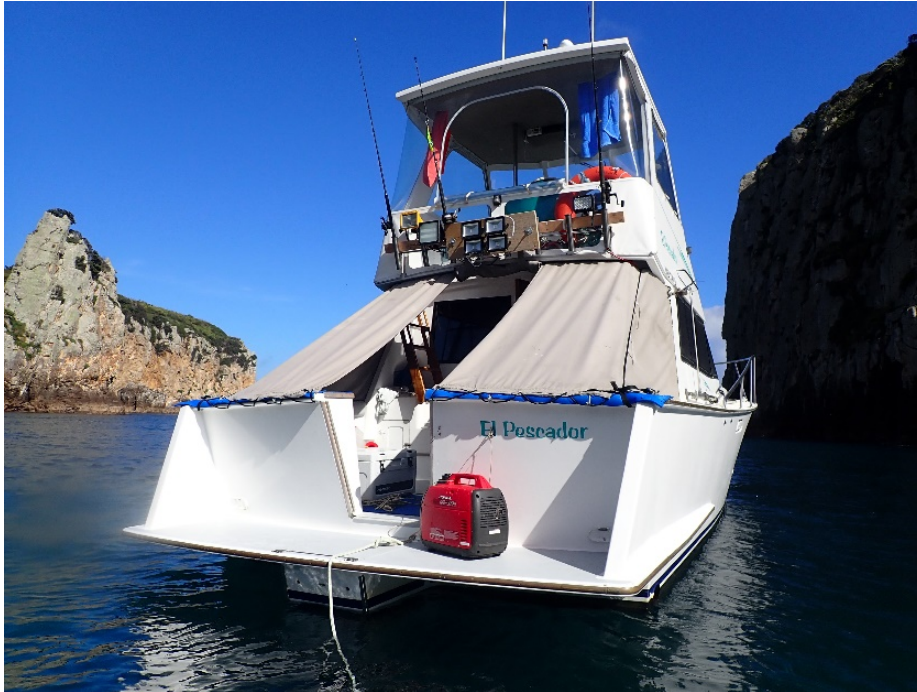
Figure 7. The El Pescador charter boat used during the lighting experiments near the Mokohinau Islands in October and November 2020. The photo shows the lighting set up, generator placement and canopy covers used to prevent birds from getting injured when striking the vessel.
